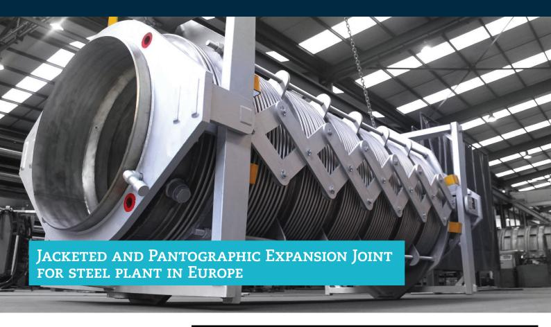
We have completed the engineering, manufacturing, testing and shipping of a Jacketed and with Pantographic Linkage Expansion Joint for one of the largest steel plants in Europe.
