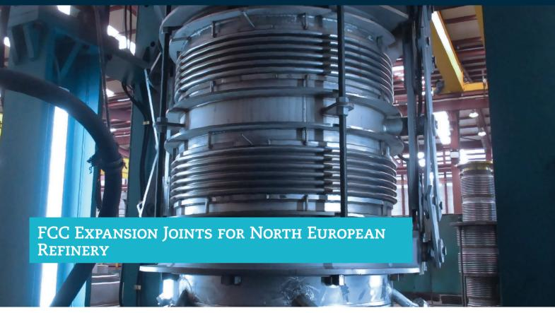
The expansion joints used in the FCCU service are exposed to high temperatures, high pressure, large movement, aggressive media and hostile environments.
